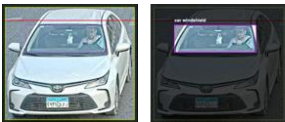
Figure 8. ROI area on car windshield with the driver wearing a seat belt
